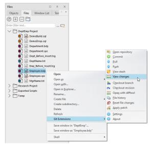
The file popup menu will include a submenu for the version control GUI that you have configured (in this case *Git Extensions*) that contains all relevant version control operations.
