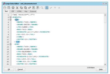
Here you can see the structure of the XML document through its syntax highlighting and folding sections. Pressing the *Parse* button will parse the XML document, and will report any errors. This requires that you have Net8 8.1 or later, and that the user has access to the SYS.XMLTYPE type or the XMLPARSER package. Pressing the *Format* button will format the XML document.
