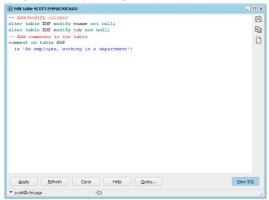
You can save the SQL to a file, copy it to the clipboard, or open it in a Command Window with the corresponding buttons at the upper right corner of the window. The *Print* button on the *File* ribbon will print the SQL. You can additionally make changes to the SQL and apply the changed SQL. After applying the changed SQL, the window will return to form mode and will refresh the table definition. Changes made to the SQL will immediately be reflected in the forms.
