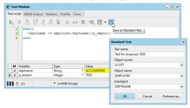
You can enter the name of the test, which will be displayed in the popup menu. You also need to enter the owner and name of the function or procedure for which the standard test will be displayed. In case of a packaged function or procedure or an object method, you also need to enter the name of the Subobject, as shown in the screenshot above.
