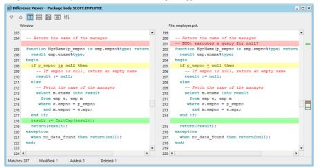
On the left you see the source from the current context. In this case the Program Window source. On the right you see the source to which it is compared. In this case the original file from the file system. The line numbers for both sources are displayed in the left margin.
