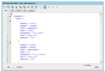
Here you can see the structure of the JSON document through its syntax highlighting and folding sections. Pressing the *Parse* button will parse the JSON document, and will report any errors. Pressing the *Format* button will format the JSON document.
