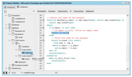
The Code Contents keep track of your current location in the source code. As you navigate through the source code, the selected item will indicate where exactly you are located.
