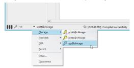
Window connections can either be pinned or unpinned. When unpinned  $(- \square)$ , the window connection will follow the main connection when the main connection is changed. When pinned  $(- \square)$ , the window connection will remain the same when the main connection is changed. To view or change the pinning of the window connection, view or click on the button in the connection status panel.
