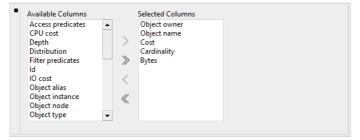
These preferences control which columns of the plan table should be displayed in the Plan Window (see chapter 6.1), and in which order they should appear.
