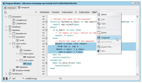
In the example above, the cursor is located at a Select statement within a Code section within an If statement within a Code section within a Function. If you move the mouse over the items of the Code Hierarchy, the corresponding source code will be highlighted. Clicking on an item will select the corresponding source code.
