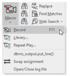
The ribbon now displays a recorder icon with a red light, indicating that you are currently recording a macro. All keyboard strokes are recorded for playback, which implies that you should not use the mouse during macro recording. By pressing F11 again, macro recording is ended. Pressing F12 will playback the macro. To repeat a macro multiple times, select the *Repeat Play* item from the *Macro* menu. The following screen will appear:
