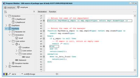
To fold a code section, press the minus sign in the left margin of the editor. To unfold it, press the plus sign in the left margin. You can also right-click in the left margin and select *Fold All* or *Unfold All* from the popup menu. If you move the mouse cursor over a folded line in the editor, the folded section is temporarily displayed in a separate pane.
