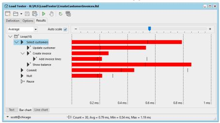
In the left pane you see the hierarchy of steps and on the right pane you can see the average time for each step, as well as a line for the minimum and maximum time.
