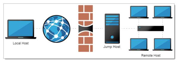
You need to access the remote hosts, but you want to limit risks and expose only the Jump Host to the internet traffic. This allows you to create strict firewall rules and to open only a single port. Therefore, it forces you to connect to the Jump Host before hopping to a remote host.
