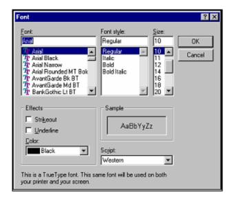
Note that the size of the font selected will be correctly reproduced only when the metafile is displayed at the size specified in the target height and width boxes on the Code page. The metafiles image created if fully resizable, so changing the size of the barcode image will also change the actual size of the font used for the text.
