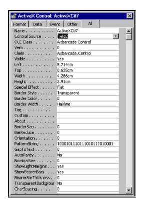
Active Barcode Component properties for a barcode image on a form or report may also be set at run-time using Visual Basic module code to modify the control's properties.
