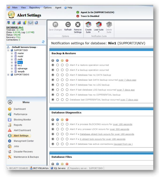
The selected severity of each notification (disable, information, warning and error) will define the dashboard color when an alert is activated.
