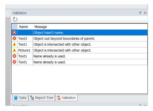
Errors and warnings can be of the following types: unnamed objects, objects with the same name, overlapping objects, objects with zero height or width, and objects that are partially or completely outside the parent object.
