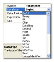
For example, for MsSqlDataConnection the parameter is of type SqlDbType :
