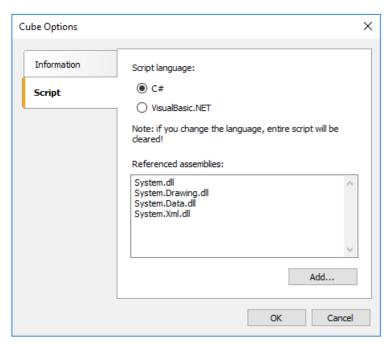
For example, if you want to use a function in your cube which was declared in your application, add application assembly (.exe or .dll) in a cube assemblies list. After that you can call the function by using namespace of your application. For example, if the following function is defined in application:
