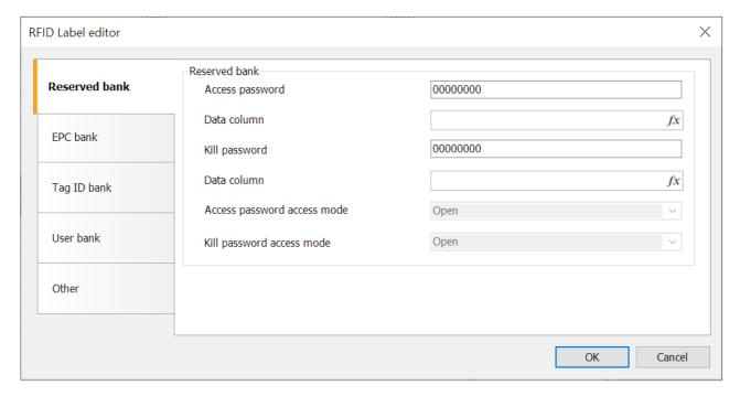
RFID tags can be created by some Zebra printers, therefore, in addition to the tag object itself, we implemented their export to ZPL. For correct export, the RFID tag must be in a single copy on the page.
