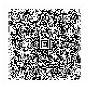
Aztec Code and combines the best ideas of 2D bar codes: MaxiCode, SuperCode, CodeOne, DataMatrix, DotCode and PDF417. Despite the patent, this development has become public domain. The coding standard is described in ISO/IEC 24778:2008.
