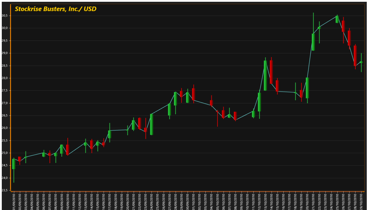
Figure 6-61. One StockSeries with Style = CandleStick. Light blue line is a PointLineSeries in the background going through all Close values.
