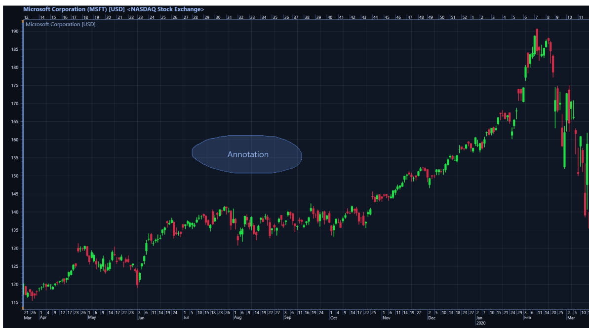
Figure 18-15. A Freehand Annotation has been drawn. A text is shown in the center of the annotation ( ShowText = true ).
