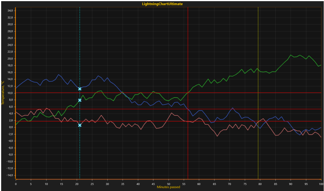
Figure 6-121. Line series cursors: Vertical point tracking cursor (cyan line and crosses), hair-cross tracking cursor (red lines) and vertical full-length cursor without tracking (yellow line)
