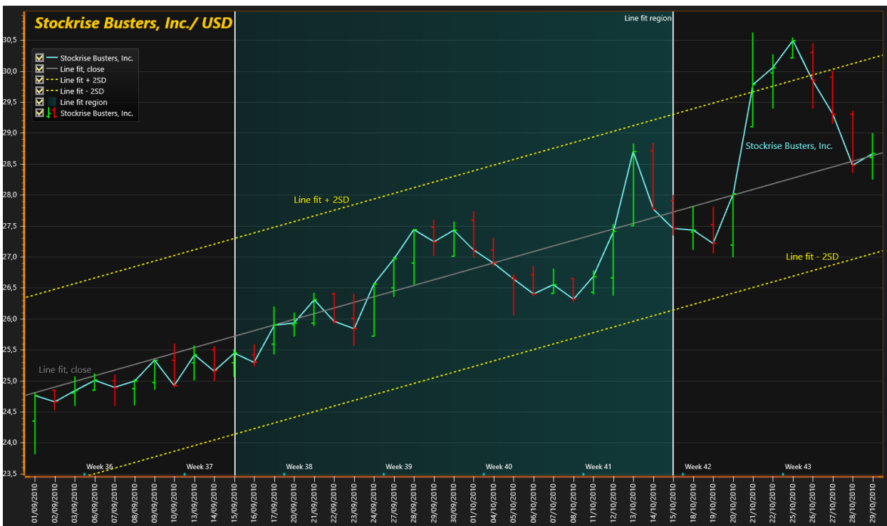
Figure 6-62. One StockSeries with Style = Bars. Line series are used for showing linear regression fit and offset of that line (2 * standard deviation). A band is used for selecting a date range for line fit.
