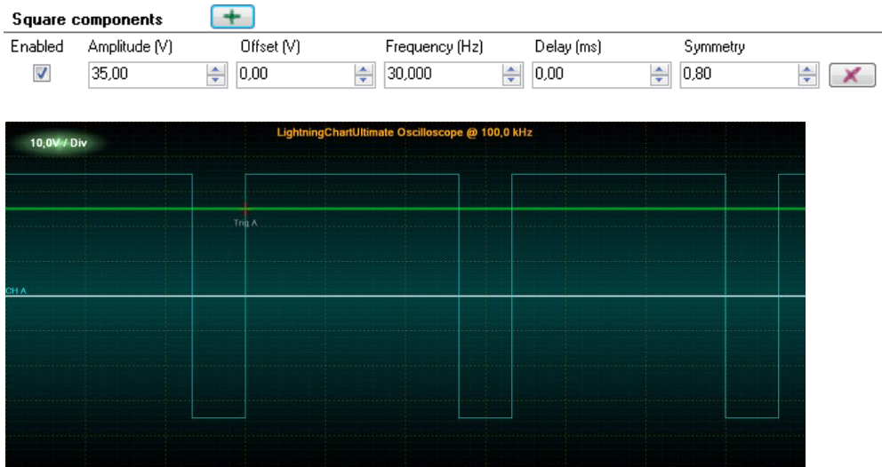
Figure 19-4. One square waveform signal, with symmetry of 0.8. Settings above.
