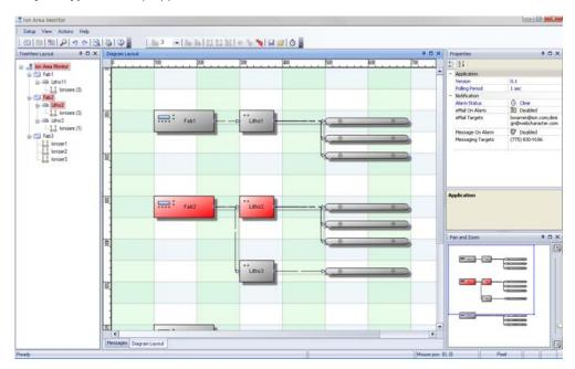
**AreaMonitor** was developed to overcome a setup and monitoring problem for ceiling emitter ionizers. Large fabrication installations could have hundreds of ionizers distributed in several buildings. These ionizers need continuous monitoring -- a malfunction could cost tens of thousands of dollars in a very short period.
