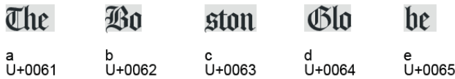
Fig. 7.3 The font report for a logotype font shows that the font contains wrong Unicode mappings. A custom code list can correct such mappings.
