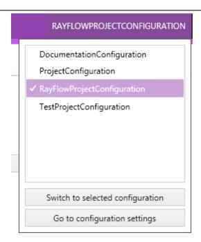
The view shows all available configurations. In the example screenshot only the default configurations are available. To add a new configuration file press the **Go to configuration settings** button located underneath the list. More regarding the configuration settings can be found in the Project chapter.
