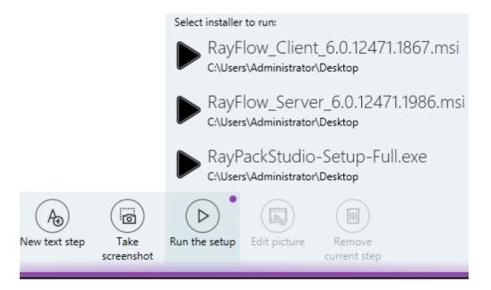
After selecting the package file that is to be installed, the package installer is initiated, and a screenshot is taken automatically. This screenshot will be used as the first step in evaluation process.
