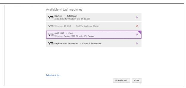
In this screen, the virtual machines that shall be used for the evaluation can be selected. Machines that have been configured but are currently not available are grayed out and marked by a warning symbol. The selected machines are highlighted as shown in the screenshot above. Click on the **Use selected...** button to use the selected machines or click on the **Close** button to return to the local machine.
