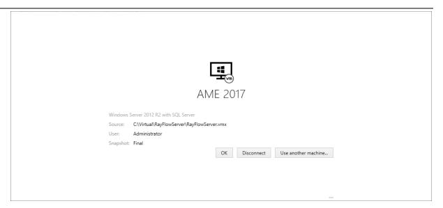
This screen can be used to either change the virtual machine, continue with the evaluation, or disconnect. Furthermore, some information about the virtual machine like path, user, and the selected snapshot are shown in this screen.
