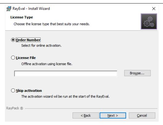
The **License Type** screen provides options to either activate the RayEval instance via order number and online activation service, by using an already prepared file (\*.license), or to skip activation for now. If the activation is skipped, it will need to be performed later when RayEval is launched. For more information on product activation at the first launch of RayEval read this section.
