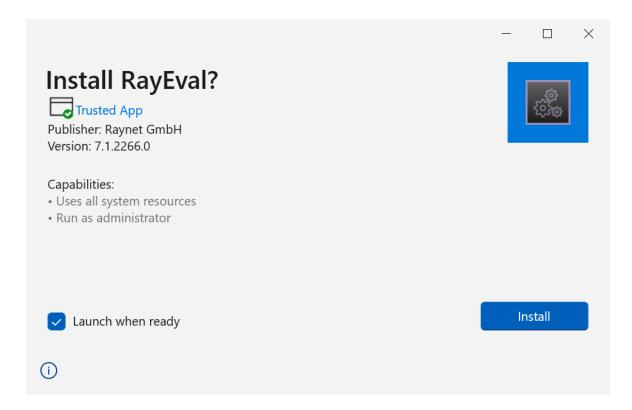
It is possible to either automatically launch RayEval after the App Installer has been closed or to decide against an automatic launch of the application by checking or unchecking the **Launch when ready** checkbox.
