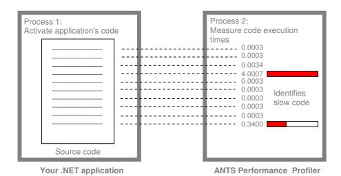
Schematic, showing how ANTS Profiler's code profiler works.
