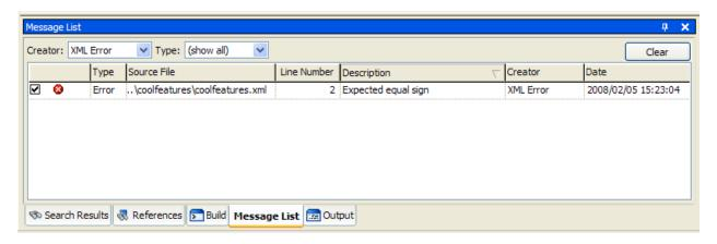
Messages are shown in tabular format with the information divided into columns. Click on a column header to sort by that column in ascending order, or click again to sort in descending order. An arrow in the column header indicates the ascending or descending sort order. Drag the column separators to resize columns.
