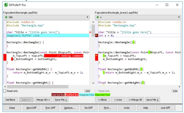
A contiguous set of the same type of differences (inserted lines or modified lines) is called a **block**. A block can be a whole line or several lines. If a particular code change to a file consists of three modified lines followed by three inserted lines, that comprises two blocks of three lines each. Operations you perform will act upon a block, a line, or the whole file.
