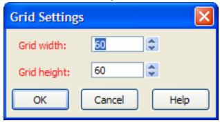
The width and height parameters are in twips (1440 twips equal one inch on the display).
