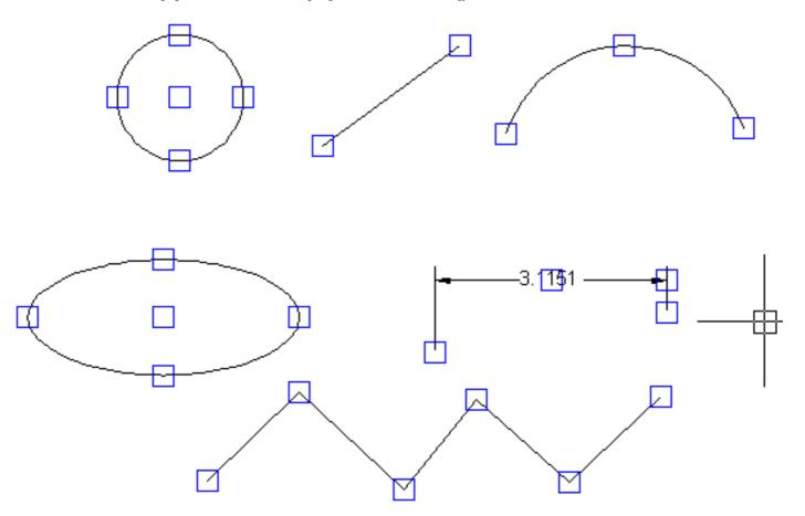
VectorDraw automatically shows the Grips on objects that are click if the EnableAutoGripOn is true. The EnableAutoGripOn property is a value representing if the mouse click will show the grips of the entities and also if the window Select command will start when the user click's to the control and there is no Entity below.
