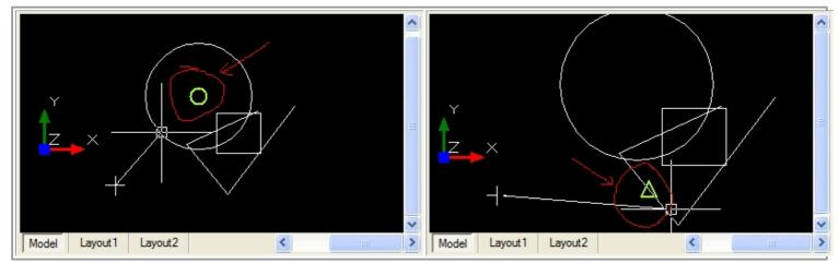
vdFC.BaseControl.ActiveDocument.osnapMode |= VectorDraw.Geometry.OsnapMode.MID; vdFC.BaseControl.ActiveDocument.osnapMode ^= VectorDraw.Geometry.OsnapMode.MID;
